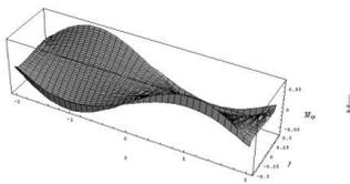
**Figure.34. Twisting moment  $\bar{M}_{xy}$  for 1<sup>st</sup> mode by LSFD [8]**
