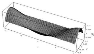
**Figure.31. Bending moment  $\bar{M}_y$  for 1<sup>st</sup> mode by LSFD [8]**
