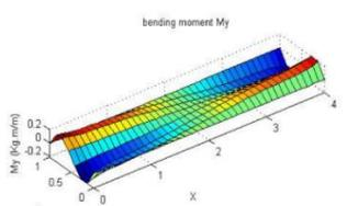
Figure 23. Bending moment  $\bar{M}_y$  for 2<sup>nd</sup> mode by ANSYS
