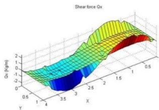
Figure 21. Shear force  $\bar{Q}_x$  for 1<sup>st</sup> mode by MATLAB
