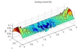
**Figure.33. Bending moment  $\bar{M}_y$  for 1<sup>st</sup> mode by MATLAB.**
