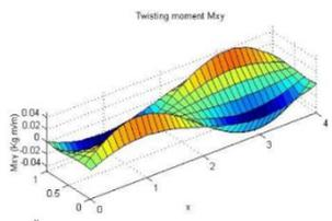
Figure 17. Twisting moment  $\bar{M}_{xy}$  for 1<sup>st</sup> mode by ANSYS
