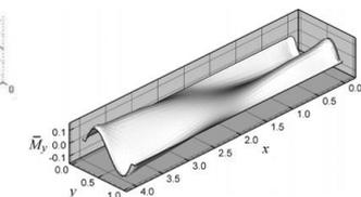
Figure 22. Bending moment  $\bar{M}_y$  for 2<sup>nd</sup> mode by LSFD [8]
