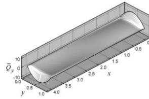
Figure 25. Shear force  $\bar{Q}_y$  for 2<sup>nd</sup> mode by LSFD [8]
