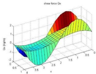
Figure 20. Shear force  $\bar{Q}_x$  for 1<sup>st</sup> mode by ANSYS.
