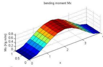
Figure 14. Bending moment  $\bar{M}_x$  for 1<sup>st</sup> mode by ANSYS
