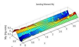
Figure 24. Bending moment  $\bar{M}_y$  for 2<sup>nd</sup> mode by MATLAB
