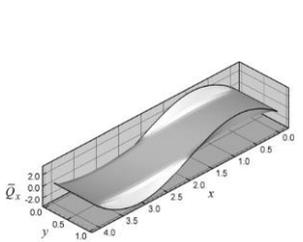
Figure 19. Shear force  $\bar{Q}_x$  for 1<sup>st</sup> mode by LSFD [8]
