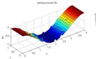
**Figure.30. Bending moment  $\bar{M}_x$  for 1<sup>st</sup> mode by MATLAB**
