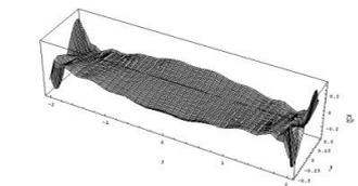
**Figure.37. Shear force  $\bar{Q}_y$  for 1<sup>st</sup> mode by LSFD [8]**
