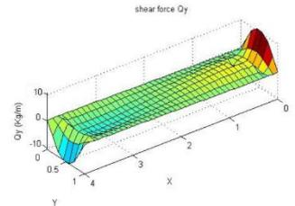
Figure 26. Shear force  $\bar{Q}_y$  for 2<sup>nd</sup> mode by ANSYS.
