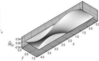
Figure 16. Twisting moment  $\bar{M}_{xy}$  for 1<sup>st</sup> mode by LSFD [8]
