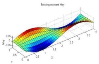
**Figure.35. Twisting moment  $\bar{M}_{xy}$  for 1<sup>st</sup> mode by ANSYS.**
