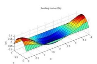
**Figure.32. Bending moment  $\bar{M}_y$  for 1<sup>st</sup> mode by ANSYS.**
