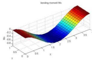
**Figure.29. Bending moment  $\bar{M}_x$  for 1<sup>st</sup> mode by ANSYS.**
