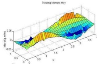
Figure 18. Twisting moment  $\bar{M}_{xy}$  for 1<sup>st</sup> mode by MATLAB.
