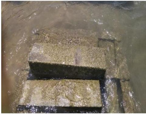
Figure 3. Beam specimens in Oman Sea environment
