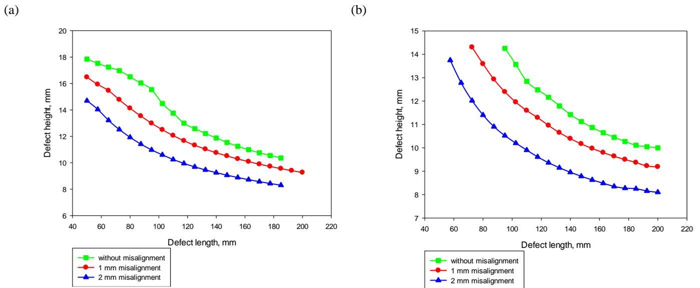
Figure 8- Tolerable defect size curve according to BS 7910- level 3B for circumferential: (a) External surface flaw, (b) Internal surface flaw
