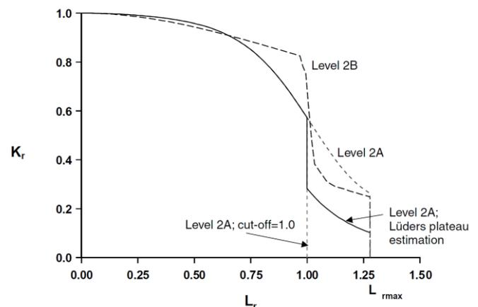
Figure 1- BS 7910 level 2 failure assessment diagram [3]
