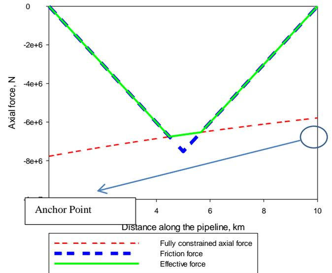
Figure 3- Effective axial force along the pipeline length
