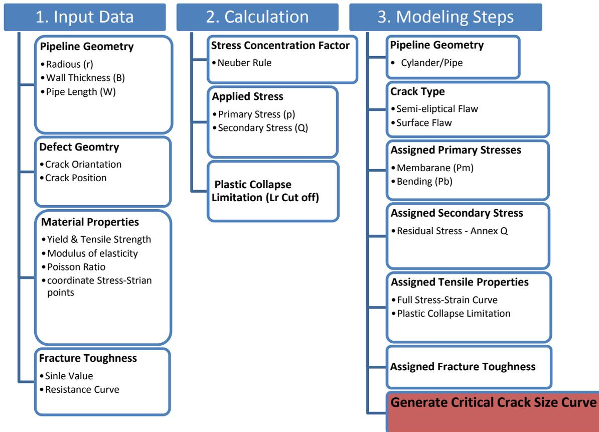
Figure 4 - Crackwise modeling and analysis sequences [16]
