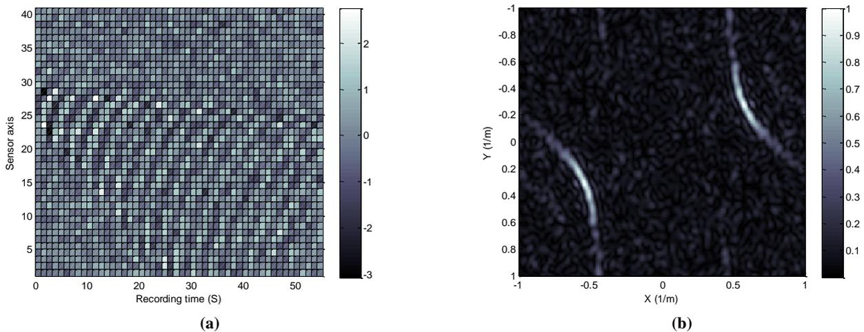
**Figure 4. (a) Magnetic wake amplitude (nT) at vessel speed 10 m/s,  $\alpha = 25^\circ$  and SNR=0 dB recorded by 40-element array sensor arrangement with  $N = 50$  and  $f_s = 0.5$  Hz (b) Normalized spectrum of the corresponding magnetic wake.**
