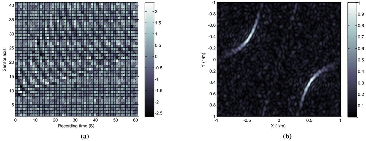
**Figure 5.** (a) Magnetic wake amplitude (nT) at vessel speed 10 m/s,  $\alpha = -35^\circ$  and SNR=0 dB recorded by 40-element array sensor arrangement with  $N = 50$  and  $f_s = 0.5$  Hz (b) Normalized spectrum of the corresponding magnetic wake.
