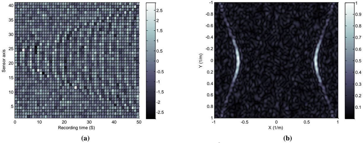
**Figure 3. (a) Magnetic wake amplitude (nT) at vessel speed 10 m/s,  $\alpha = 0^\circ$  and SNR=0 dB recorded by 40-element sensor array arrangement with  $N = 50$  time-steps and  $f_s = 0.5$  Hz. (b) Normalized spectrum of the corresponding magnetic wake.**
