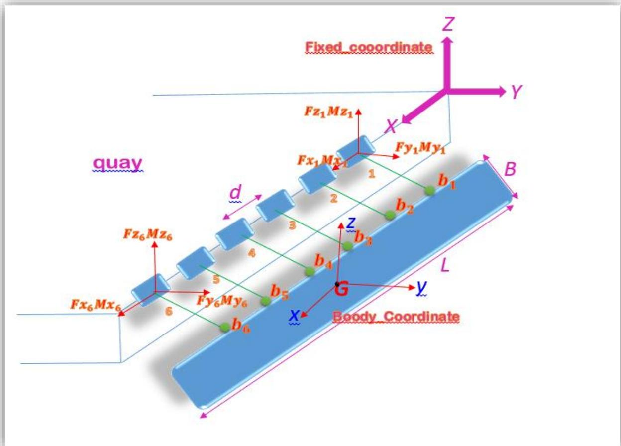
Figure 6 - A schematic of the moored ship connected to 6 MoorMaster units
