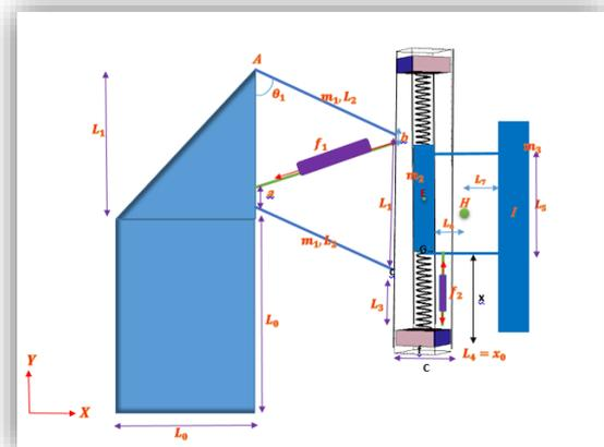
**Figure2- Extracted dynamics modeling of MoorMaster**
