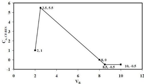
Figure 2:  $C_{a,CF-RES}$  as a function of reduced velocity [3]
