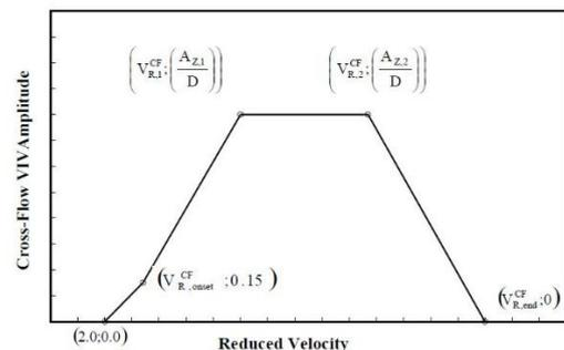
Figure 1: Cross-flow response model generation principle [4]
