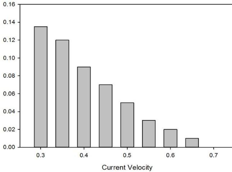
Figure 4: The current velocity probability by Weibull
