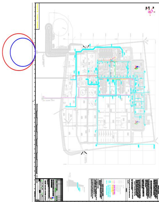
Area basin used for buoy mooring, single buoy, For LPG jetty, Max. Radius: 265m, min. Radius: 203m
