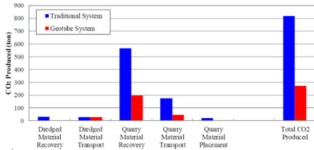
Fig. 4) CO<sub>2</sub> produced from the different parts of breakwater construction operations
