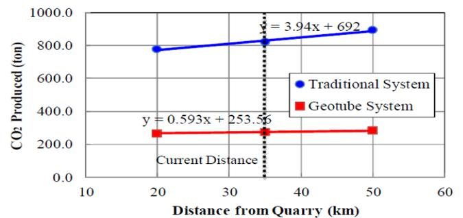
Fig. 6) CO<sub>2</sub> emissions based on a change in the distance from quarry
