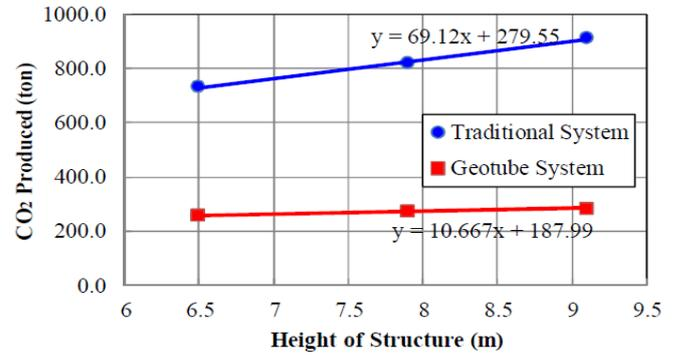
Fig. 5) CO<sub>2</sub> emissions based on a change in the size of constructed breakwater
