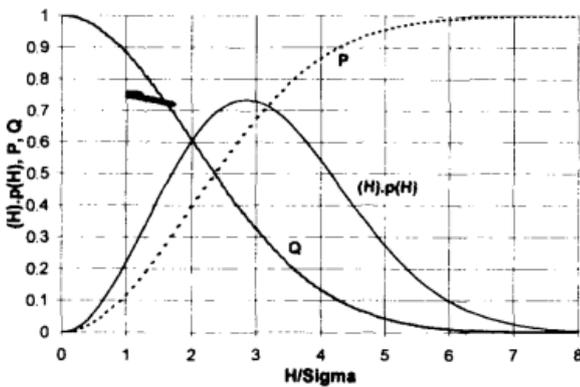
Figure 3 - Riley wave height distribution
