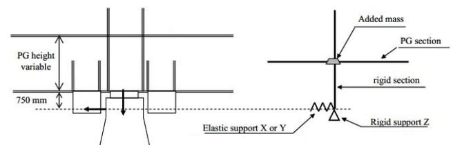
Figure 18– sample of the support connection with neoprene
