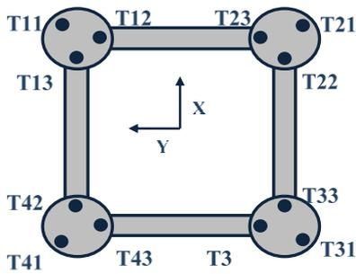
Figure 2: schematic arrangement of tendons
