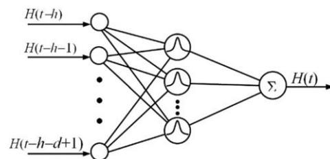
Figure 2: Structure of Radial Basis Function Neural Network [31]
